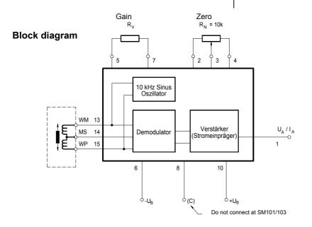
Between Pin 5 and Pin 8 the demodulated signal can be measured 0 V means plunger in midposition
