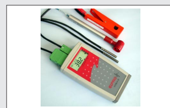
Application: monitoring fresh air 1x sensor for air velocity Part No. 3264-D 1x current clamp Mini2 Part No. 3268 2x NTC probes -50..140°C Part No. 3090-L10
