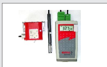
Application: clean room 1x differential pressure +/-50Pa Part No. 3260-L 1x humidity and temperature Part No. 3088-A 1x cable 1 meter Part No. 3216-L01 1x mounting plate Part No. 2804-SE1
