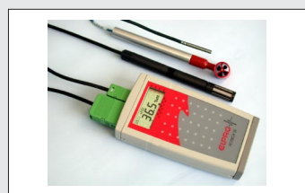
Application: recording climatic data 1x hygroclip sensor Part No. 3088-A 1x extension 1m Part No. 3216-L01 1x sensor for air speed Part No. 3264-D 1x NTC probe -50..140°C Part No. 3090-L10
