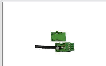
Connector for sensor connection with 4 pin terminal (2x NTC) Part No. 2540-P4 with 5 pin terminal (2x 4..20mA) 2540-P5 with 7 pin terminal (2x DC) 2540-P7
